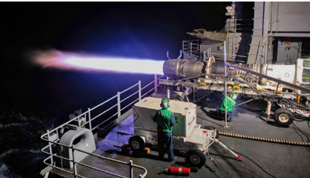
Sailors assigned to USS George H.W. Bush (CVN 77) test a jet engine cell on the ship's fantail. CharLES is reducing the time and cost it takes to simulate the aerodynamics inside an aircraft's engine and troubleshoot problems.
